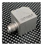
The GVT10S-TC is a general purpose cube shaped triaxial IEPE accelerometer for the measurement of broadband vibration in a wide range of vibration test applications, its small size and low mass make it an ideal all rounder. With a tapped base on two sides it provides flexible mounting options.
