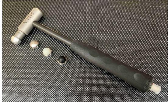
The VTH5KN is a general purpose IEPE Impact Hammer range offered by Kemo Ltd.
