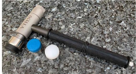
The VTH50 is the largest of the heavyweight general purpose IEPE impact hammers offered by Kemo Ltd and provides a maximum range of 50,000N of impact force.
