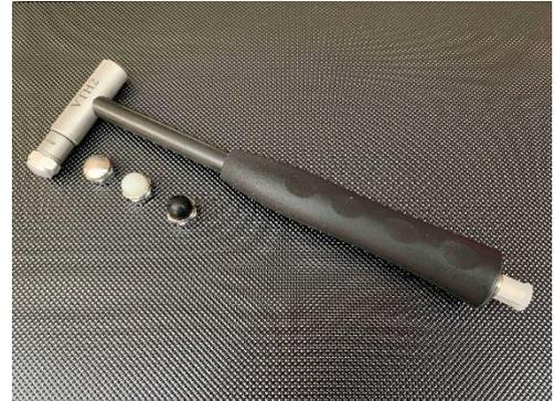
The VTH2KN is a mid-range general purpose IEPE Impact Hammer range offered by Kemo Ltd. With a range of 2000N and a sensitivity of 2.5mV/N it is well suited to a wide range of structural testing applications from lightweight to slightly stiffer testing work.
