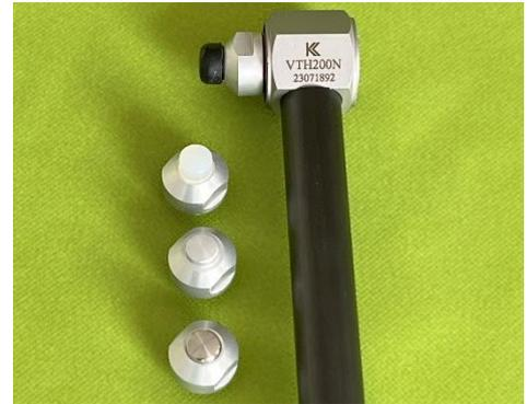
The VTH200 is a lightweight general purpose IEPE Impact Hammer range offered by Kemo Ltd.
