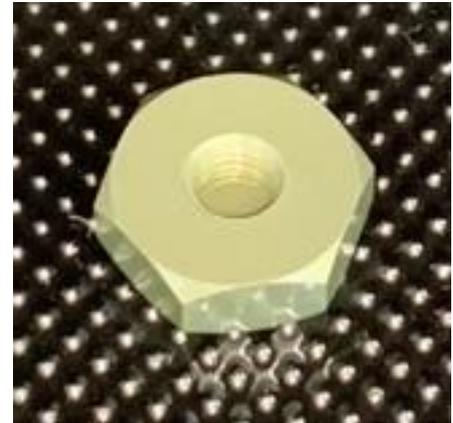
The KMISO-ADH is an adhesive mounting base for use with accelerometers and other sensors requiring surface mounting. It features an aluminium body which has been hard anodised to provide electrical isolation from the mounting surface. This solution solves issues of earth loops causing interference in data signals from sensors.
