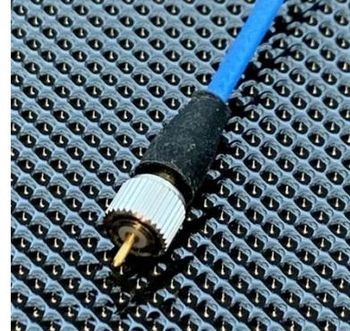
The 10/32UNF Microdot plug connector is industry standard in applications such as accelerometers, pressure sensors and other similar test and measurement sensors. Its compact size and secure thread fitting are well suited to sensor applications.
