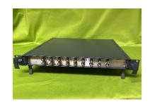
The 9X-CI is a 9 channel IEPE and charge signal conditioning unit, housed in a compact and rugged 1U high 19" rack mount chassis. Featuring DC power input, it can be used via the supplied mains DC adaptor or via a field-based DC supply such as battery.
