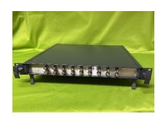
The 9X-C is a 9-channel charge amplifier/signal conditioning unit, housed in a compact and rugged 1U high 19" rack mount chassis. Featuring DC power input, it can be used via the supplied mains DC adaptor or via a field-based DC supply such as battery.
