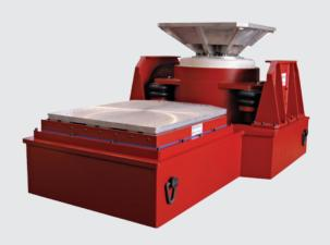
Water cooled shaker bodies are completely sealed, making them ideal for both clean room and hazardous environments.
