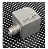
The GVT10S-TC is a general purpose cube shaped triaxial IEPE accelerometer for the measurement of broadband vibration in a wide range of vibration test applications, its small size and low mass make it an ideal all rounder. With a tapped base on two sides it provides flexible mounting options.
