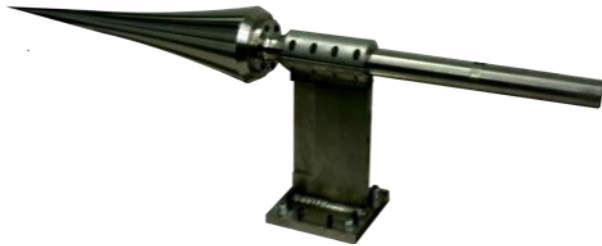
Figure 11: NASA Langley 93-10 flared cone model, on bench (left) and installed in M6QT (right)
