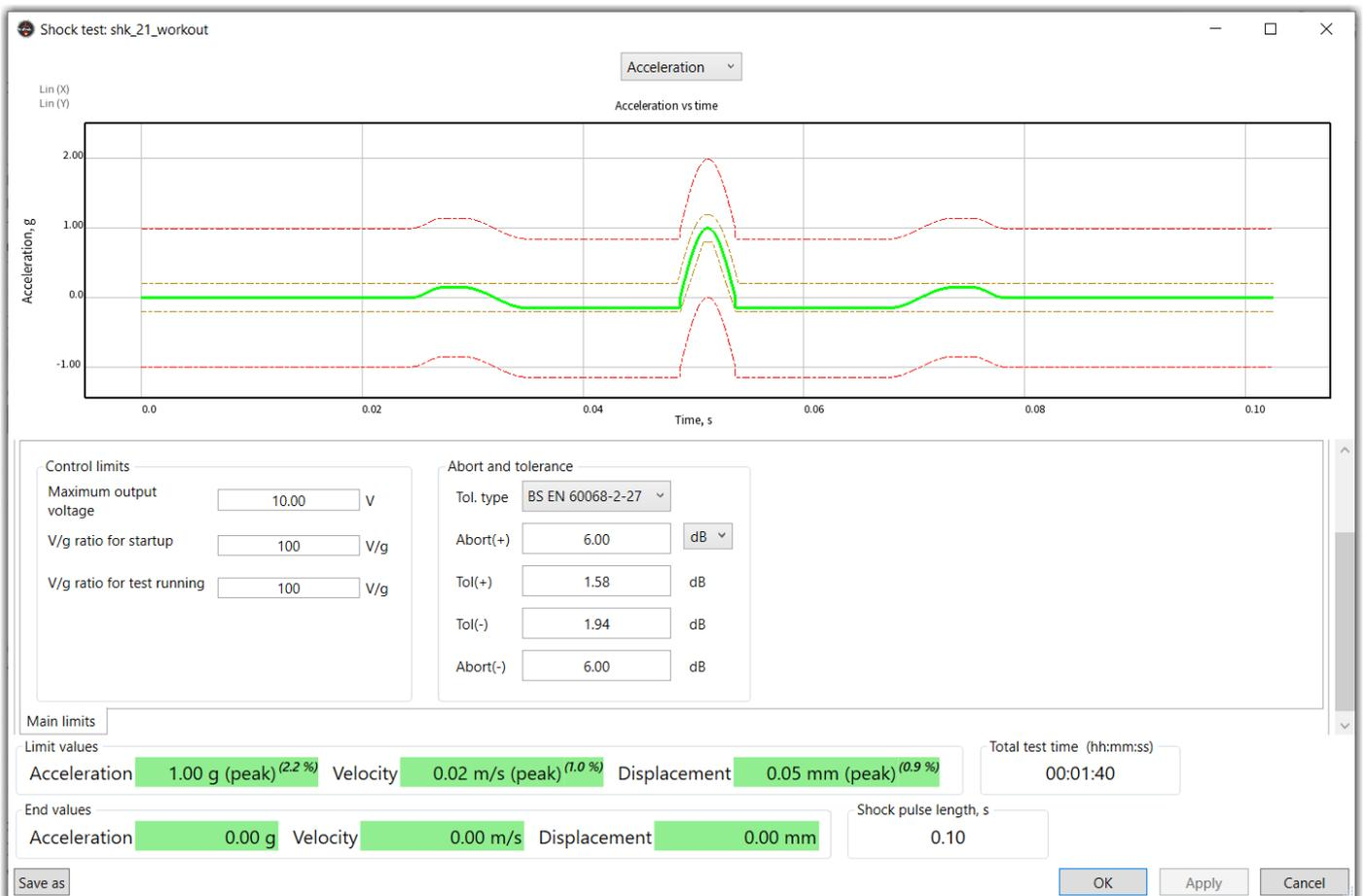
5. Table – the tolerance levels of the “Shock pulse power” deviation from task, taking into account the level specified in the schedule, are specified according to the table entered by the user. The abort levels are user defined.
