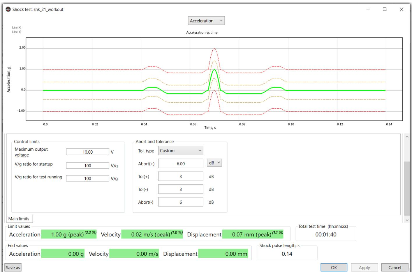
2. MILSTD 810 – the levels of shock pulse power deviation in reference to the task level are specified as per MILSTD 810 (US Ministry of Defense standard). The abort levels are user-defined
