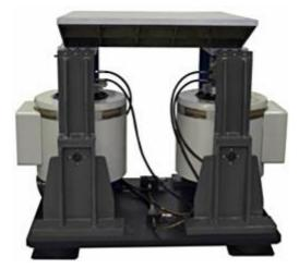
RL-C21 and RL-C25 vibration control systems apply computation of transfer-function matrix to maintain the phase and amplitude in multishaker tests, through control of shakers interaction and non-linearity of the vibration set.
